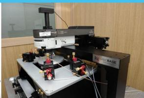
**Xper-PC**'s 3-probe measurement using a high performance 2-channel sourcemeter unit provides a variety of photocurrent information, helping you obtain such information more easily by displaying detailed photocurrent differences in a large area in a form of high quality 2D maps.
